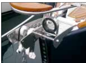
Bow bracket integrated with bow anchor fitting.
