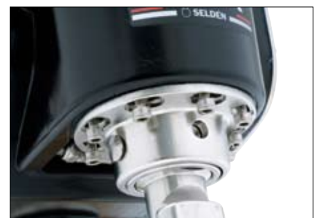
Adjustment screws enable the Furlex housing to be aligned precisely.
