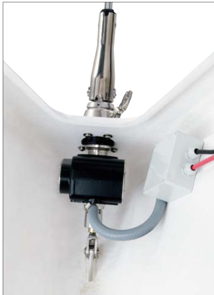
Through-deck installation of a Furlex 200E. The connection box is water-tight.
