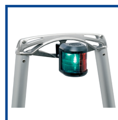
The bridle wire is secured in a slot on top of the bridle support. All prepared for navigational lights.
